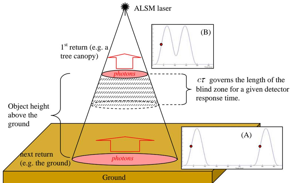
**Figure 2.** The “dead time” effect. Two hypothetical return pulses from a single transmitted pulse are shown. (A) The discriminator triggers on the leading edge of each pulse when they are sufficiently separated. (B) If the second return overlaps the first, the discriminator fails to detect the second return. For a 10 nanosecond pulse duration and a single-channel detector, the dead time corresponds to a distance of roughly 3 m. (Slatton, et al., 2007).
