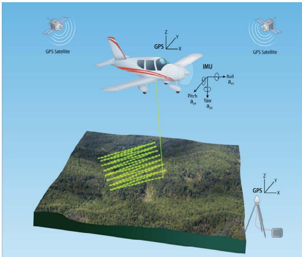
**Figure 1.** Schematic diagram (Carter, et al., 2007) of a small-footprint, discrete-return ALSM unit. ALSM systems are generally comprised of four major hardware components: (1) a scanning laser emitter–receiver unit, (2) differential global positioning systems (GPS receivers on the aircraft and on the ground), (3) a highly sensitive inertial measurement unit (IMU), and (4) an onboard computer for data capture and storage.
