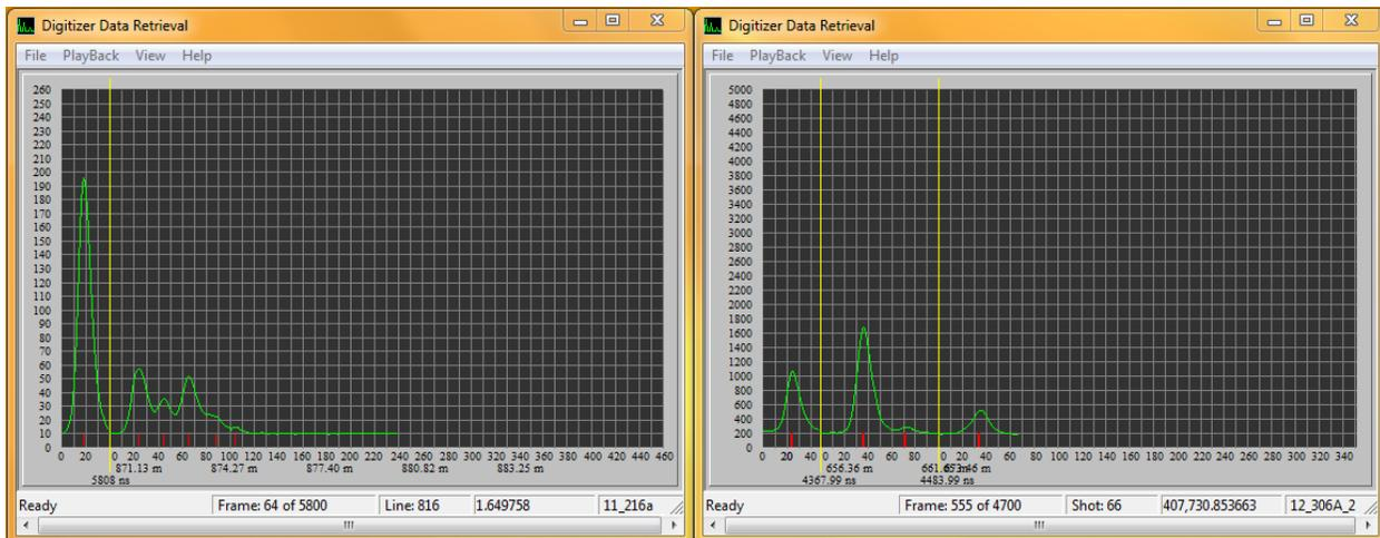
**Figure 4.** 8 and 12 bit digitized waveforms as displayed by the Digitizer Data Retrieval (DDR) software.
