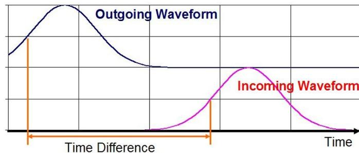
**Figure 2.** Pulsed laser time of flight ranging principle.
