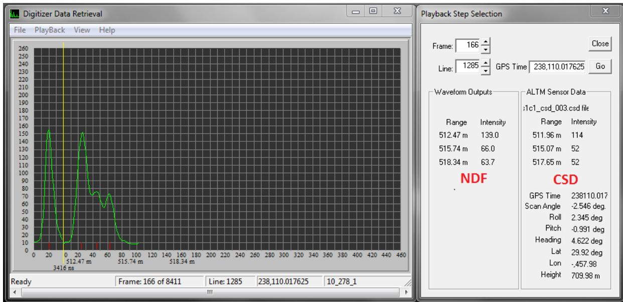
**Figure 6.** Optech’s Digitizer Data Retrieval software displaying waveform and associated CSD data.
