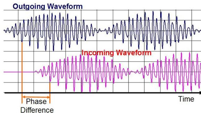
**Figure 1.** Amplitude modulated continuous laser phase difference ranging principle.
