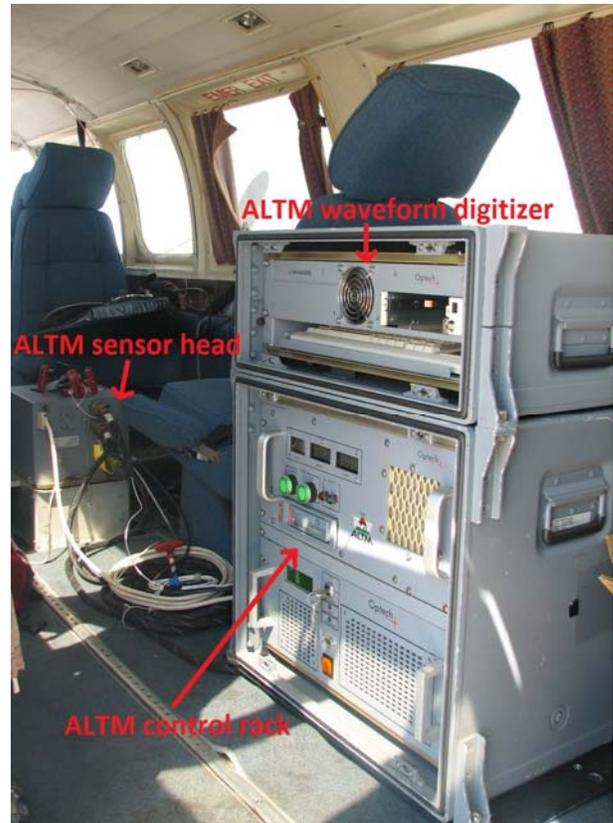
**Figure 5.** The Gemini ALTM system and 8 bit digitizer
