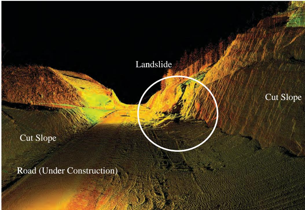
**Figure A-19: Point cloud of a rockfall on newly cut section for a highway. (Courtesy of Oregon DOT).**
