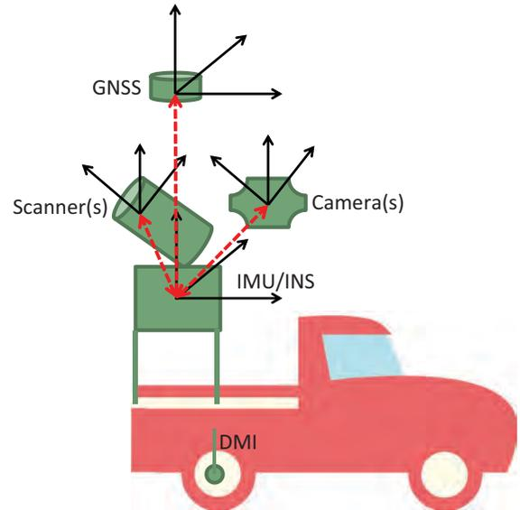
**Figure 8. Lever arm offsets to MLS components.**
