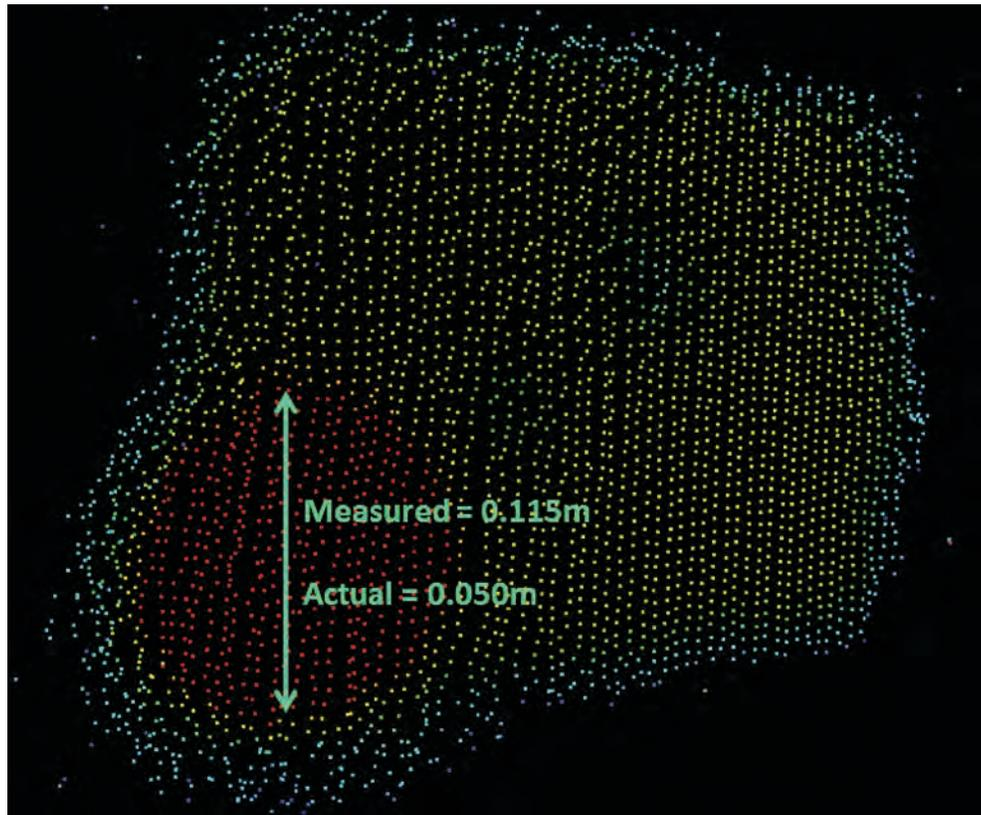
**Figure A-24: Blooming (i.e., enlargement) of a flat 5cm retro-reflective target (red).**
