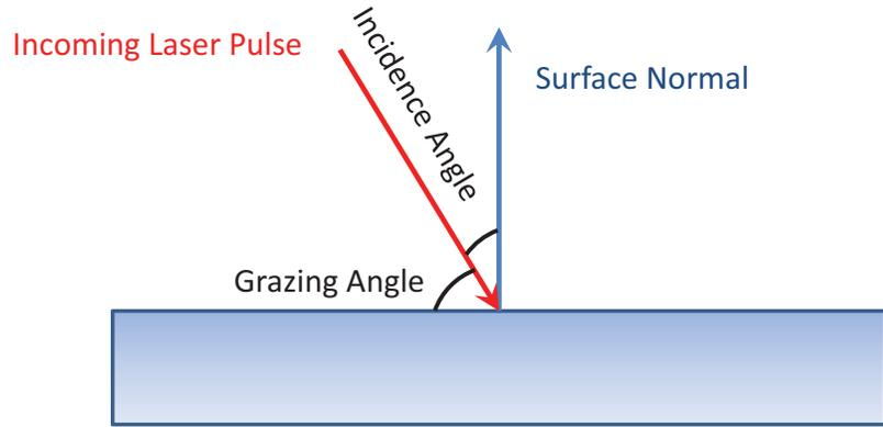
Figure G-2: Terminology for scanning geometry.
