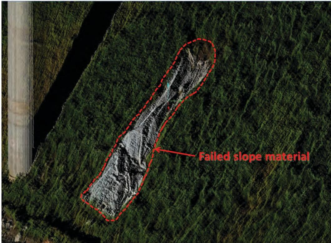
**Figure A-18: Static scan of a surficial slope failure along highway embankment at the US 20 Pioneer Mountain to Eddyville re-alignment project in Oregon. (Note that the failure scarp is covered by a white tarp to prevent sediment from entering nearby water).**
