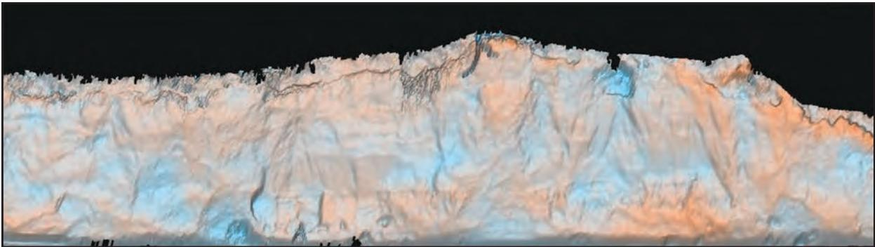
**Figure A-21: Time series change analysis for the Johnson Creek landslide along Highway 101 in Oregon obtained through “stop and go” scanning. Orange indicates erosion and blue indicates accretion and seaward movement.**
