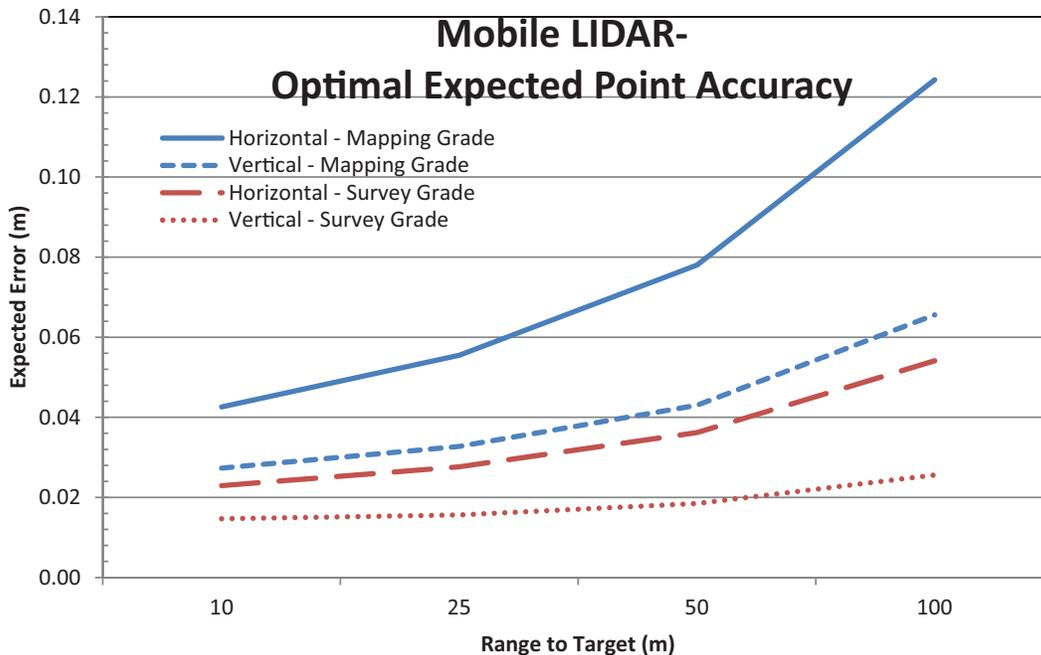
**Figure 9. Minimum expected horizontal and vertical errors under ideal conditions (site independent, optimal incidence) for typical mapping and survey grade MLS.**
