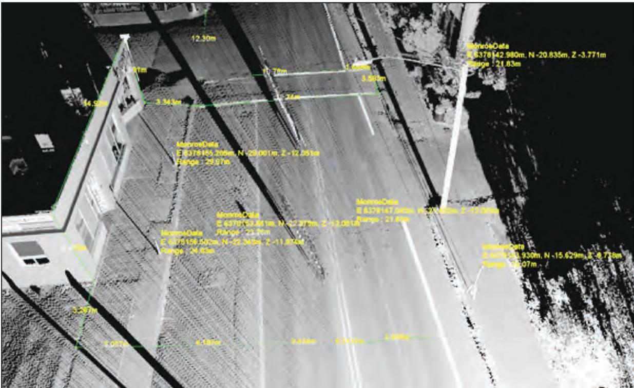
**Figure A-12: Linear measurements and point coordinates in a point cloud (static scan).**
