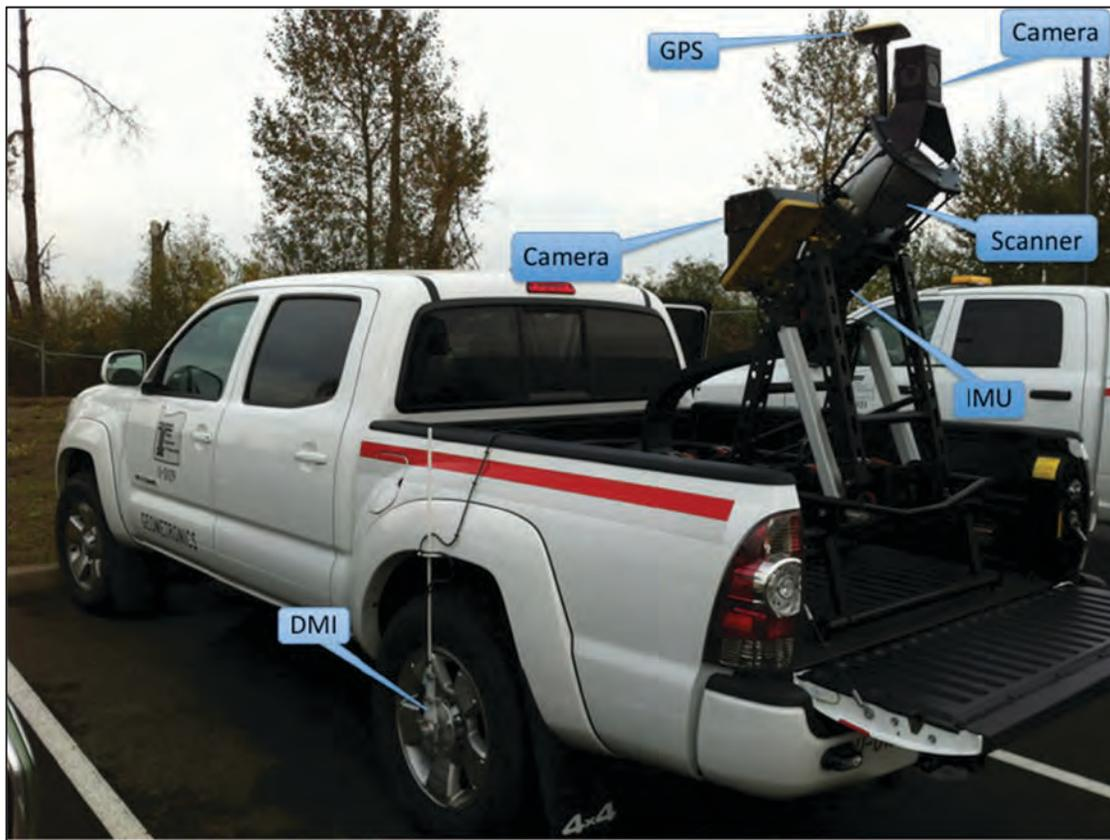
**Figure A-7: MLS system components (Topcon IP-S2 HD system operated by Oregon DOT).**
