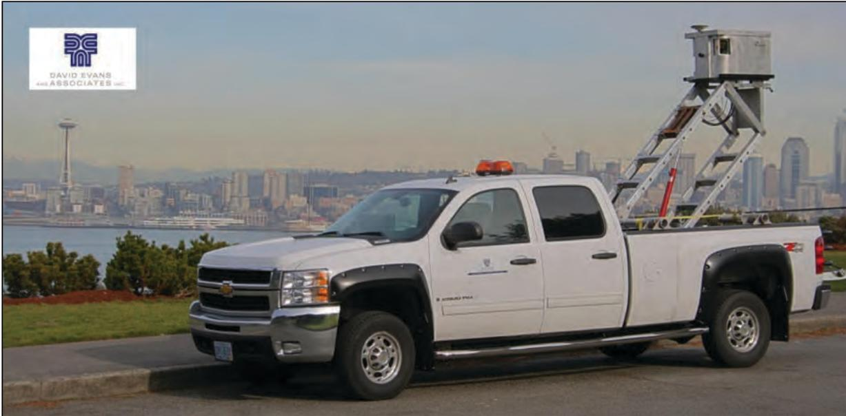
**Figure A-6: Example of a MLS system (TITAN, courtesy of DEA).**
