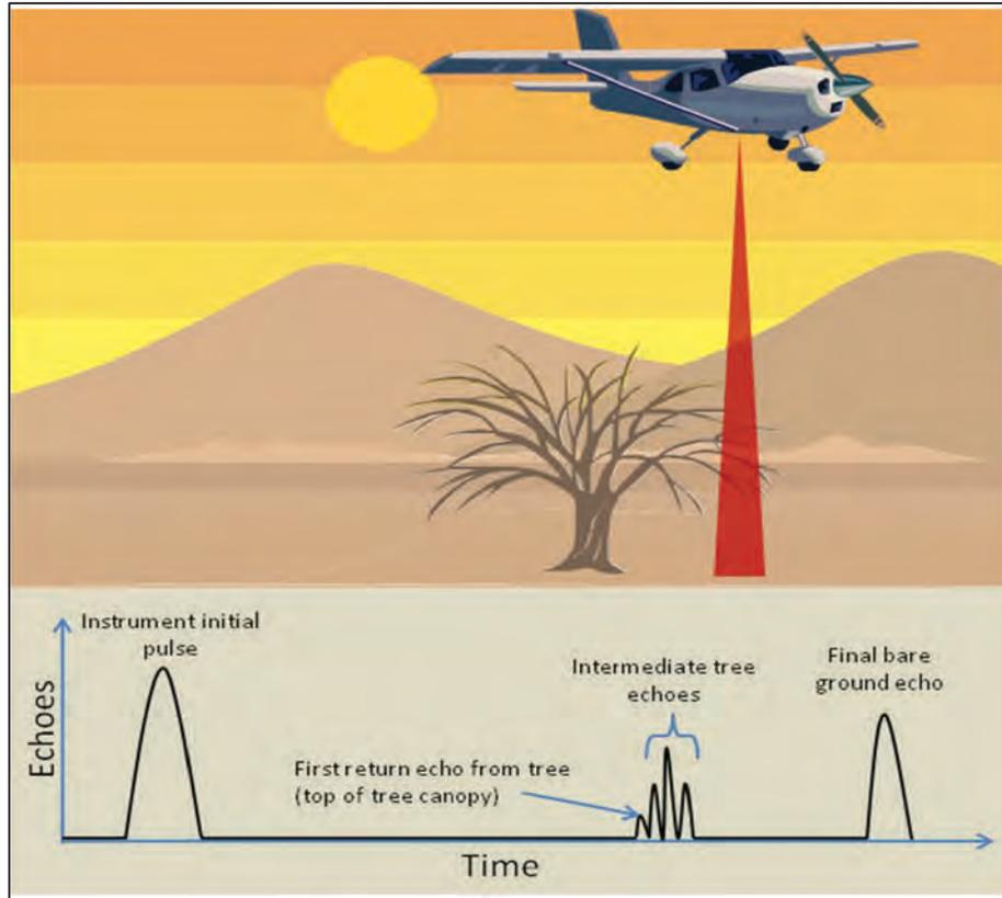
**Figure A-1: Example illustrating concept of multiple returns from a single LIDAR pulse.**
