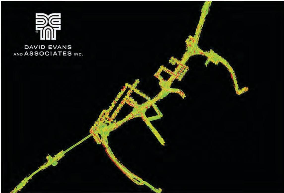
**Figure A-13: Plan view of a section of MLS data obtained for several arterial roads for the Columbia River Crossing Project, a comprehensive industrial, residential, and infrastructure redesign centered on the I-5 Bridge crossing the river. (Courtesy of DEA).**
