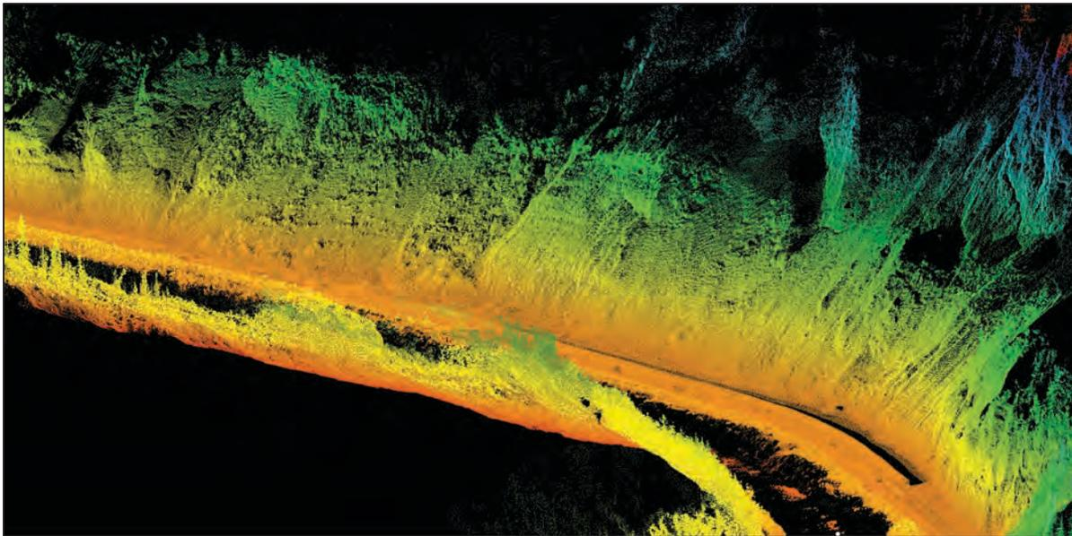
**Figure A-20: Point cloud for MLS data obtained for slope stability assessment on the Parks Highway near Denali National Park, Alaska.**
