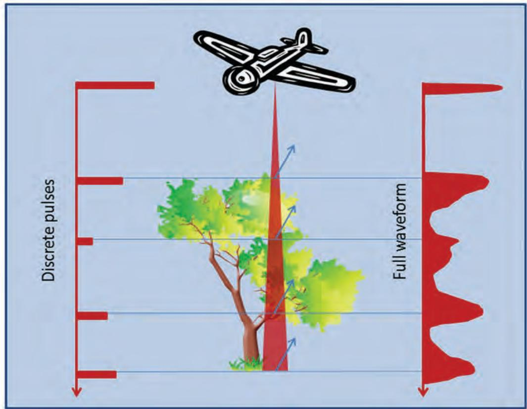
**Figure A-4: Discrete pulses vs. full-waveform returns.**
