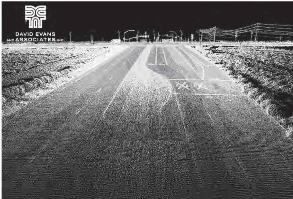
**Figure A-3: Grayscale, intensity-shaded image of mobile LIDAR data, showing painted lines and other features. (Courtesy of DEA)**
