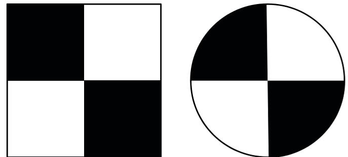
Figure 11. Examples of patterns for survey targets.
