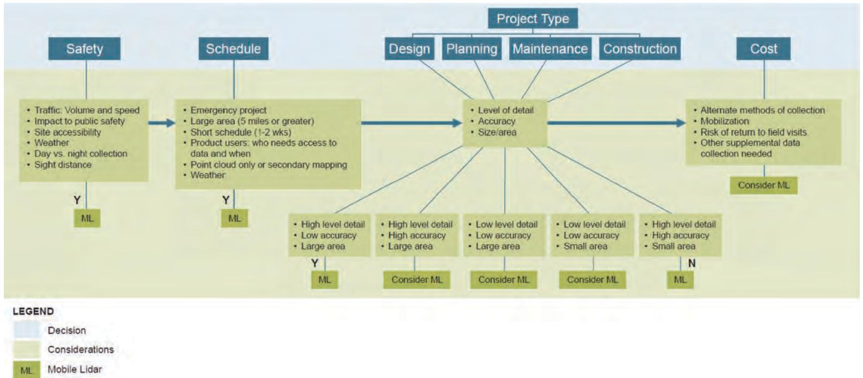
Figure 4. Decision flowchart to determine when mobile LIDAR use is appropriate for a project.
