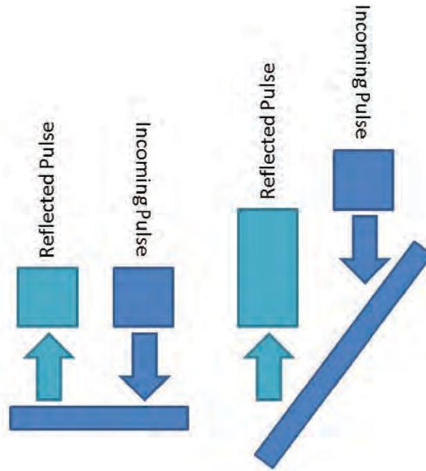
**Figure A-5: Increase of pulse width on oblique surface.**
