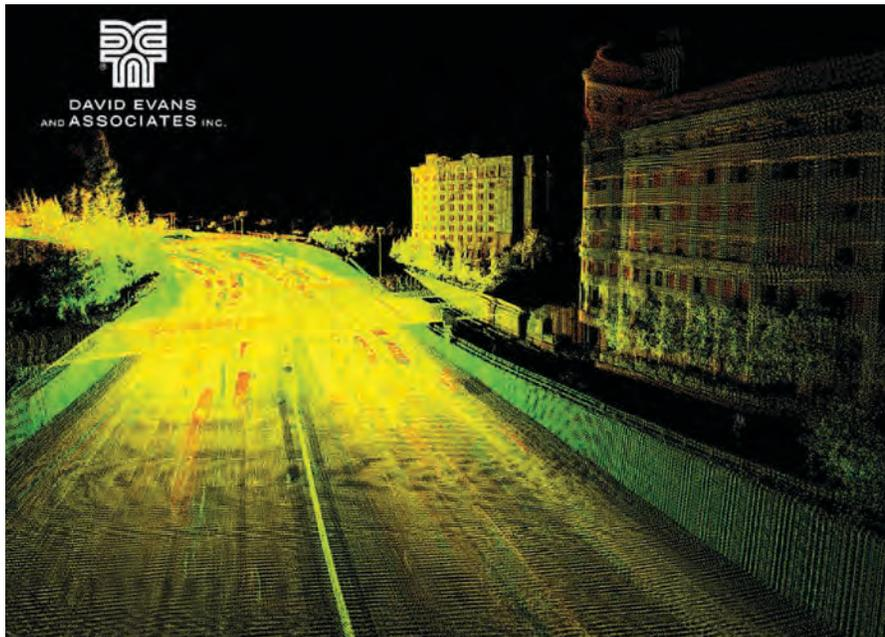
**Figure A-15: Mobile LIDAR data of a section of the I-5 corridor in Sacramento, CA (Courtesy of DEA).**
