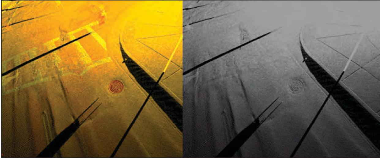
**Figure A-2: Painted street markings and manhole cover can be better distinguished in the intensity return colored image on the left. (Data from a static scan).**
