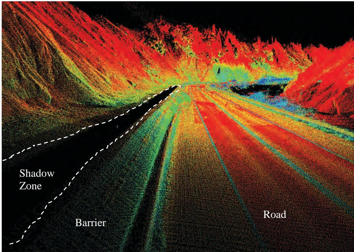
**Figure F-2: Shadows in the point cloud created by obstructions (courtesy of Alaska DOT).**
