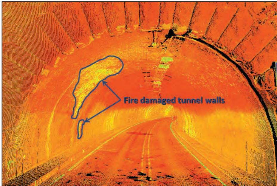
**Figure A-17: Close examination of the intensity-shaded point cloud (static scan) shows additional, minor damage to concrete in a tunnel in Oregon. (Courtesy of Oregon DOT).**
