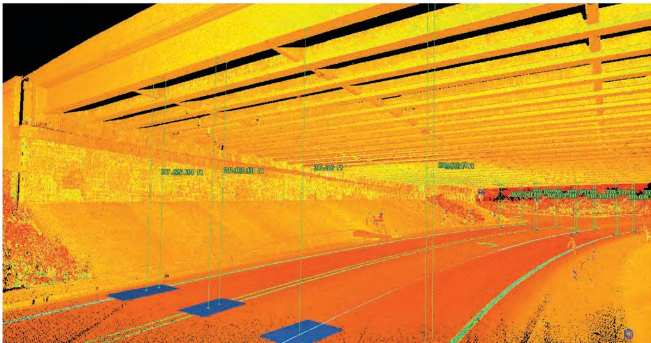
**Figure A-14: Clearance values measured perpendicular to roadway surface using a static scan point cloud (Courtesy of Oregon DOT).**
