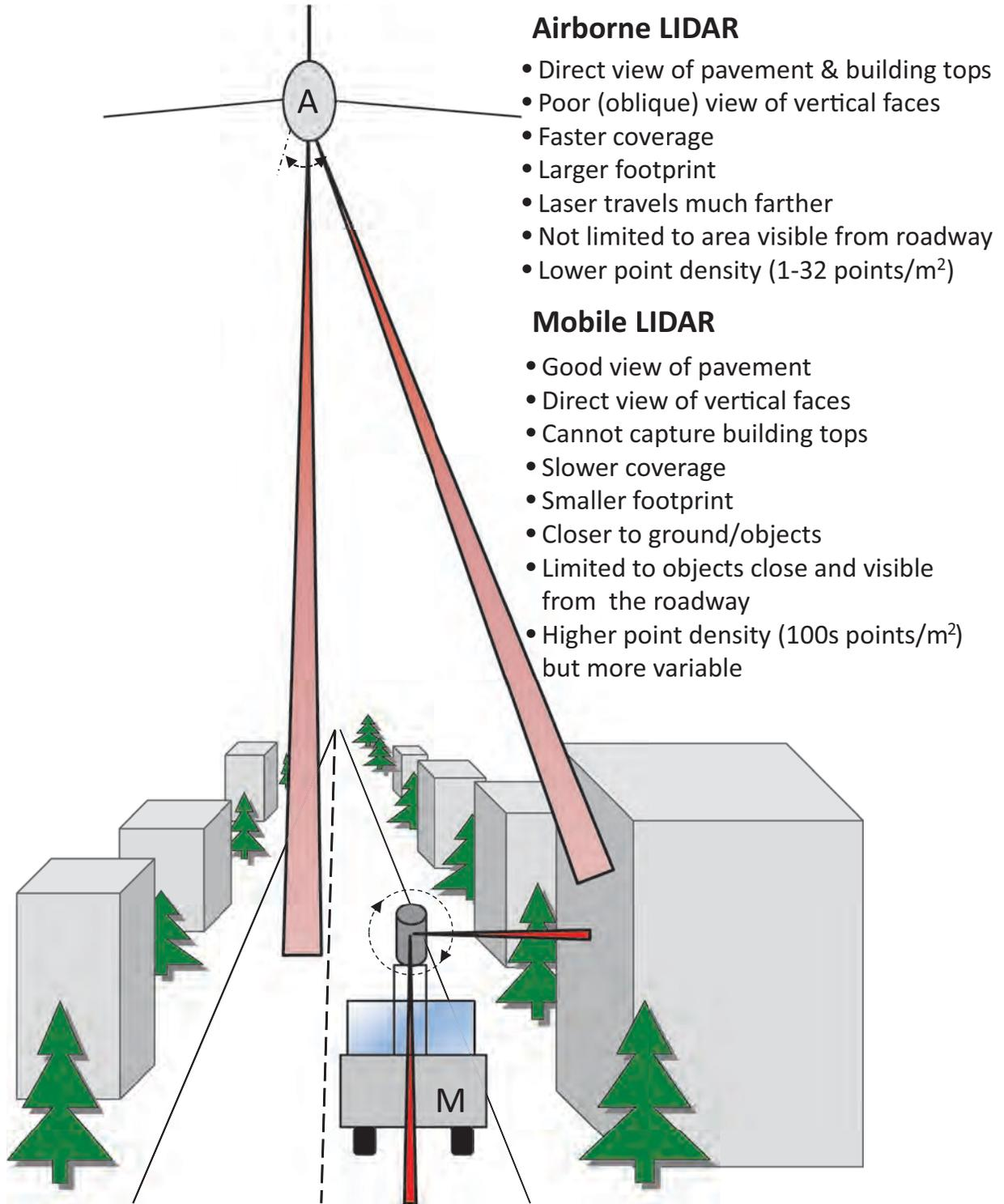
**Figure A-10: Comparison of Airborne and mobile LIDAR systems.**
