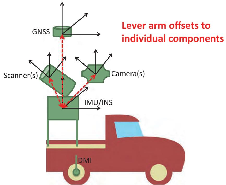
Figure G-3: Lever arm offsets to mobile LIDAR components.
