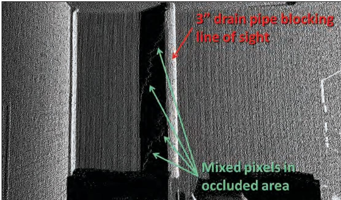
**Figure A-25: Mixed pixels appear in an area occluded from the scanner’s line of sight.**
