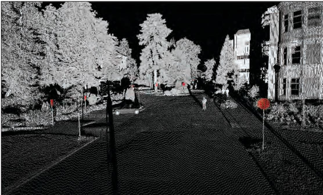
**Figure A-22: Reflective signs (red) extracted from a static TLS point cloud at the Oregon State University campus.**
