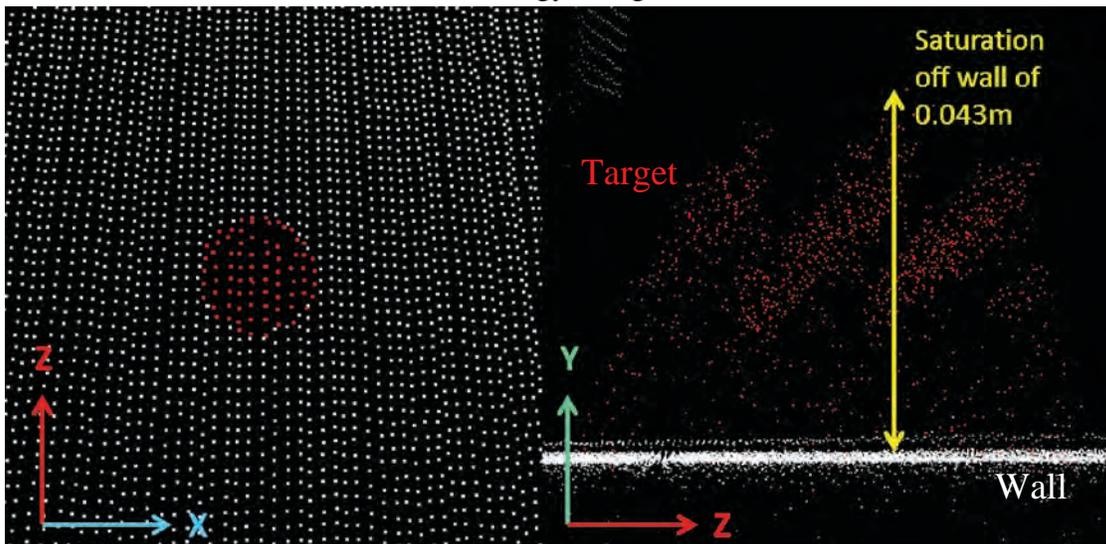
Figure A-23: Extreme case of Saturation of a flat, 5cm retro-reflective target (red) is seen as the target extending 4cm off of the wall. Left: Straight on view (down on Y-axis). Right: side view along plane of wall that target is affixed to (along X-axis).
