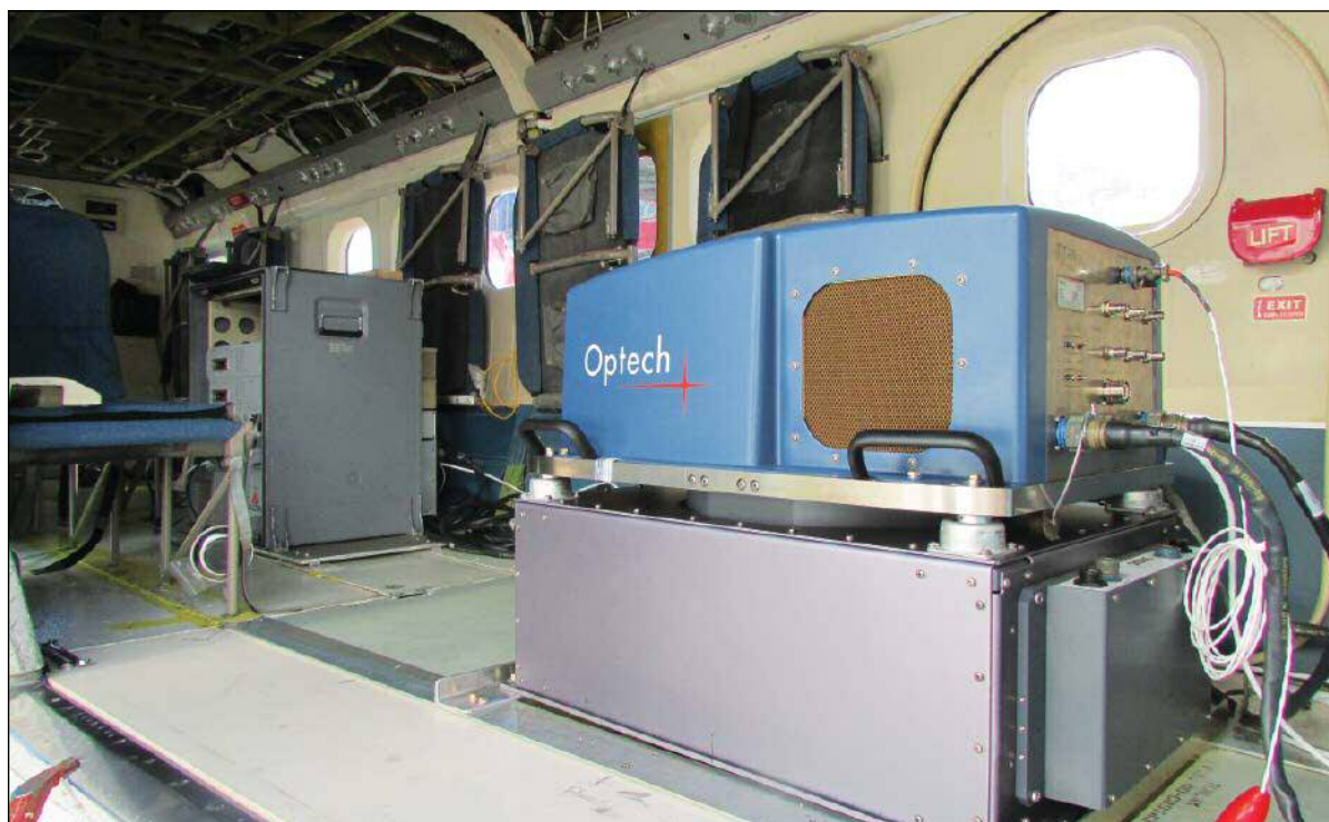
The Titan multispectral airborne laser scanner unit aboard a Twin Otter aircraft.
